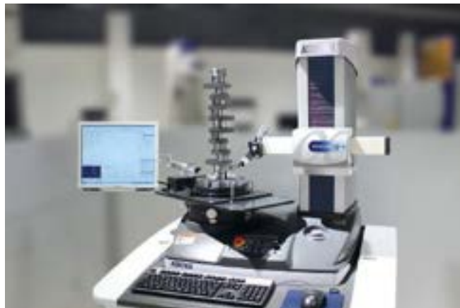
Measuring crankshaft using designated jig tool
