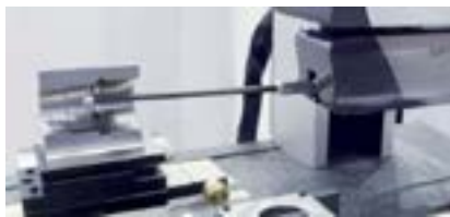
Attaching 100mm High rigidity offset arm.
